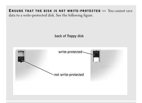
**TRY ANOTHER FLOPPY DISK** — Insert another disk to eliminate the possibility that the original disk is defective.
