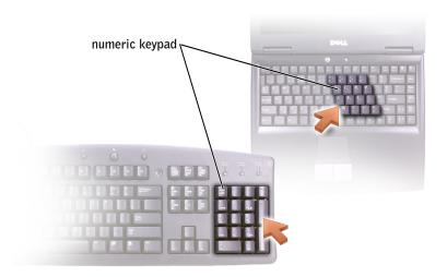
**HINT:** When you connect an external PS/2 keyboard or PS/2 keypad to the computer, the integrated keypad is disabled.
